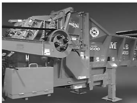
Wood Hog — Torque Limiter Torque Limiter located in driven sheave on mill shaft. Morbark 2600 - 7600 Wood Hogs 200 - 1200 hp 47,000 - 277,000 lb. in.
